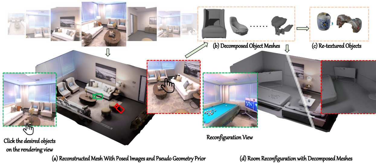
Figure 1. Indoor scenes consist of complex compositions of objects and backgrounds. Our proposed method, Total-Decom , (a) performs 3D reconstruction from posed multiview images, (b) decomposes the reconstructed mesh to generate high-quality meshes for individual objects and backgrounds with minimal human annotations. This approach facilitates such applications as (c) object re-texturing and (d) scene reconfiguration. For additional demonstrations, please refer to our supplementary materials and videos.
